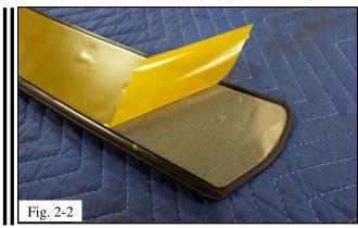
(d) While keeping the bumper protector aligned, lower the part in place. Pull small sections of the backing (Fig. 2-2) while pressing the part onto the vehicle until you have removed all of the backing and the part is secure.
