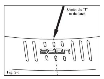
(c) Hold the bumper protector about ½" above the surface of the bumper and align the center of the "I" on the bumper protector to the center of the latch on the rear lift gate (Fig. 2-1).
